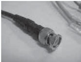
Figura 2.4. Cable coaxial con conector BNC
