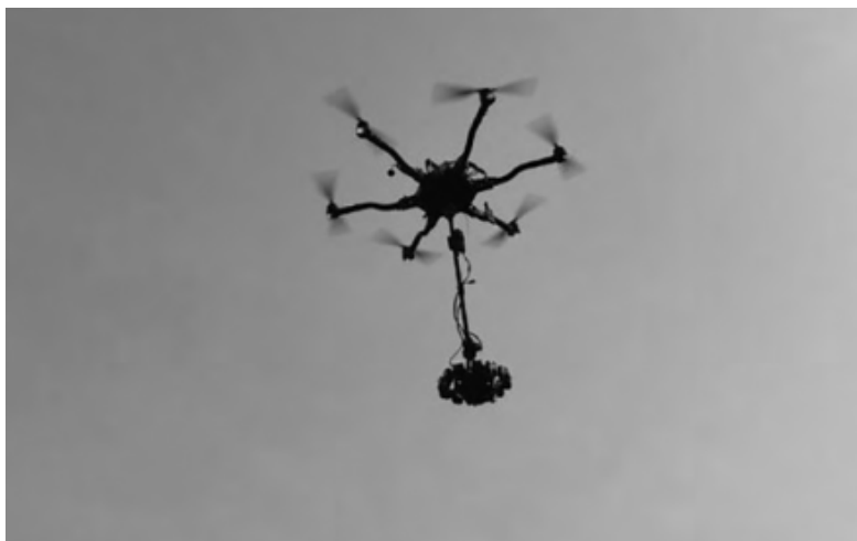
Figure 5 – With the modified three-axis gyroscope stabilizer and the United States Freefly six-axis aircraft
