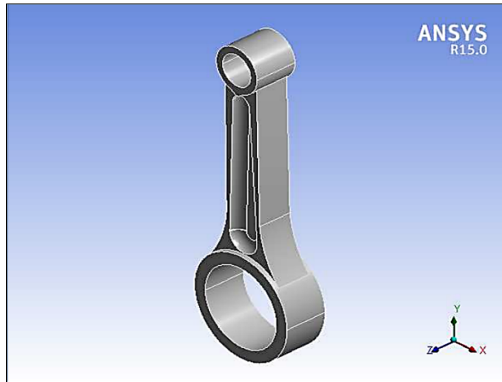
Figure 1 Geometric design of the connecting rod, with standard measurements
